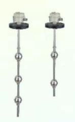
A magnetic float moves up and down on probe immersed in a liquid. The float energizes the hermitically sealed sensors, which change from NO to NC otherwise as the float-passes them.
