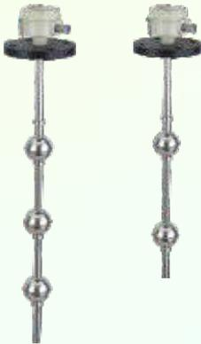
A magnetic float moves up and down on probe immersed in a liquid. The float energizes the hermitically sealed sensors, which change from NO to NC otherwise as the float-passes them.
